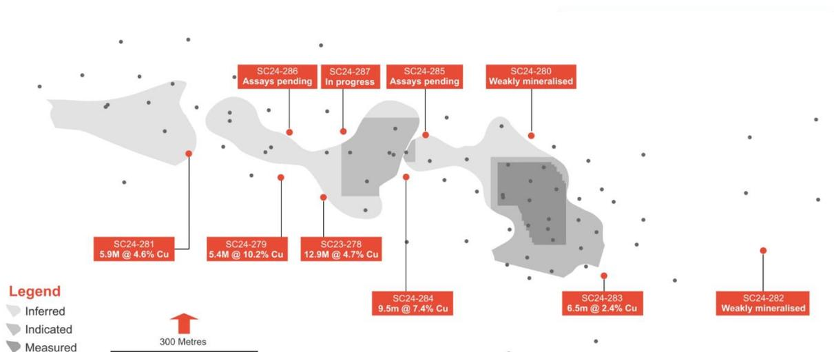
**Figure 2: Plan of the Johnny Lee Lower Copper Zone at the Black Butte Project as of March 2024, showing current and past drill pierce points (red and black dots respectively) and resource domains (shades of grey)**
